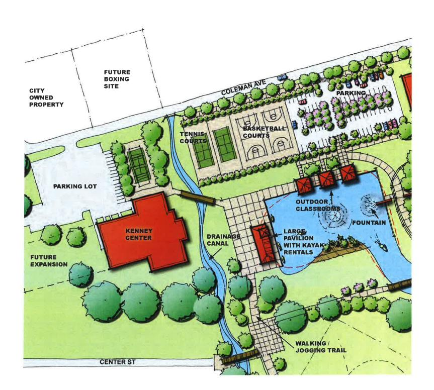
Located at the Northwestern corner of the site near the Kenney Center is the proposed re-shaped pond. This new configuration is envisioned as a pedestrian promenade with the pond shape more architectural with a concrete bulkhead, railing and lighting.
