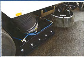
VACUUM AND BRUSH REMOVAL OF DEBRIS
