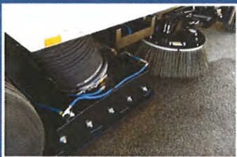
VACUUM AND BRUSH REMOVAL OF DEBRIS
