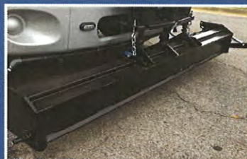
POWERFUL MAGNET TO COLLECT FERROUS MATERIAL
